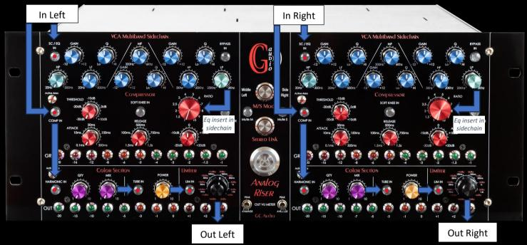
This is the default mode when you power on the. An analog processor with two completely independent channels. In this mode, you can simultaneously process two tracks independently. As the device has many functions, it is necessary to understand its routing, which prioritizes dynamic processing above all. Please consider the following diagrams:
